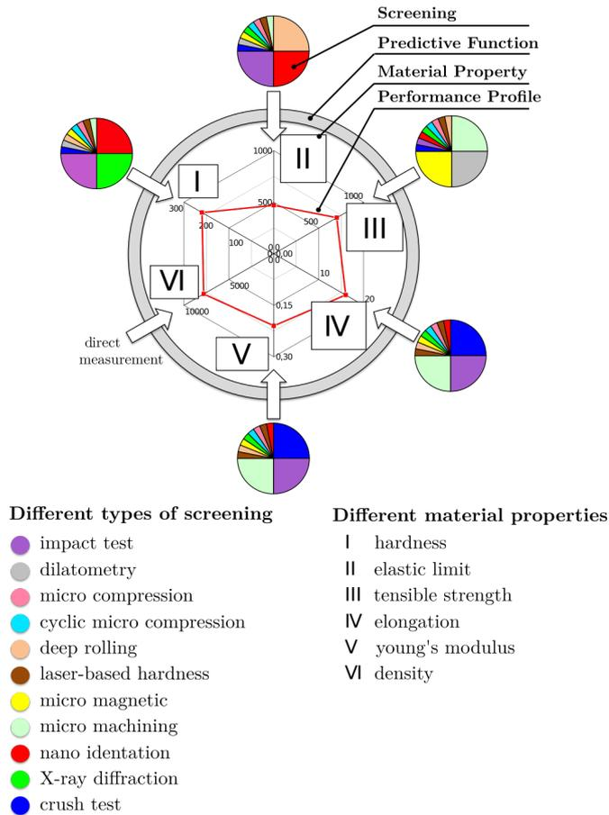
Fig. 2: Possible types of screening data & material properties
