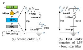
Fig. 1. RF receiver with filters – LNA: Low Noise Amplifier, LO: Local Oscillator, LPF: Low Pass Filter, ADC: Analog-to-Digital Converter
