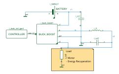
Fig. 7. Buck-boost converter system overview
