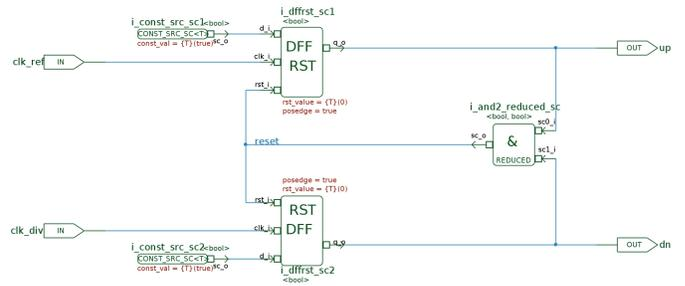
Fig. 6. Phase Frequency Detector (PFD) without a delay element
