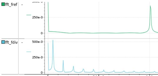
Fig. 4. FFT of PLL faulty behavior
