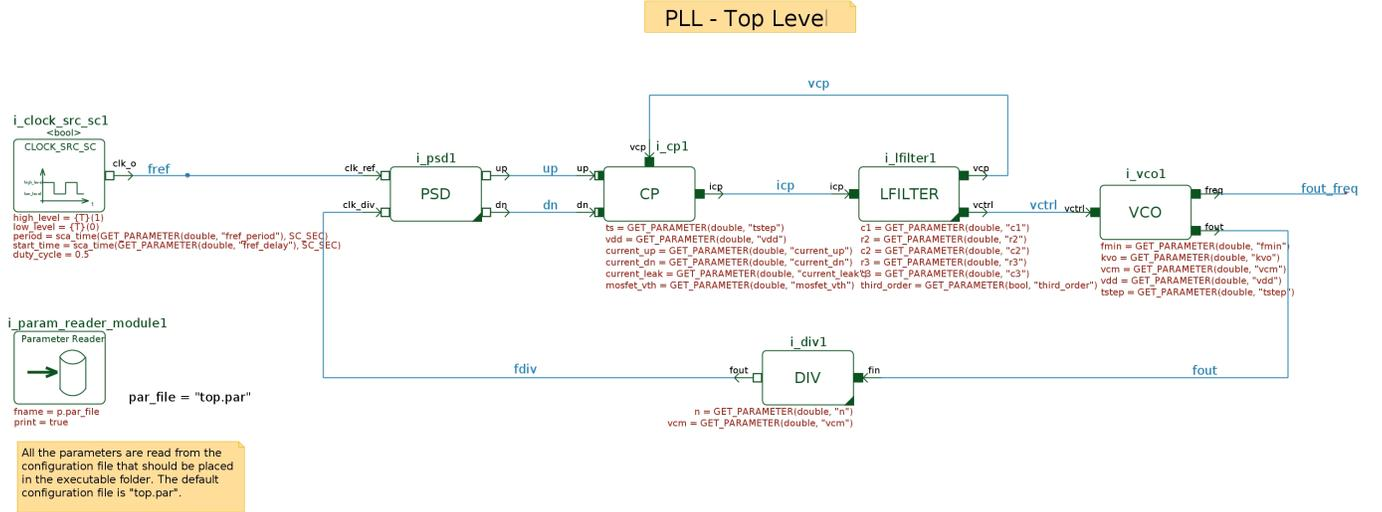
Fig. 1. PLL Top Level Diagram
