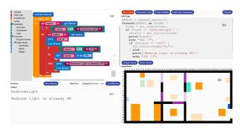
Figure 1: Screenshot of the programming application interface. (a) Blockly UI panel (translated to English); (b) Code panel; (c) Output panel (translated to English); (d) 2D graphical view of the smart home.
