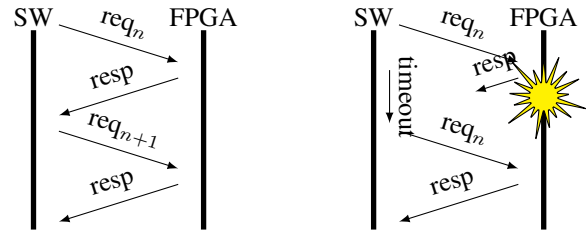
Fig. 4. Sequence diagram of the communication protocol.
