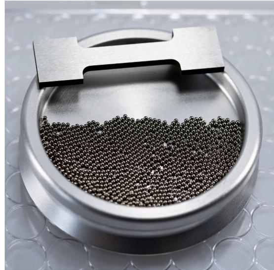
Fig. 1. Comparison between tensile test specimen and spherical micro samples (of same mass) ©Jan Rathke
