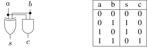
Fig. 1. Half adder logic diagram and its truth table.
