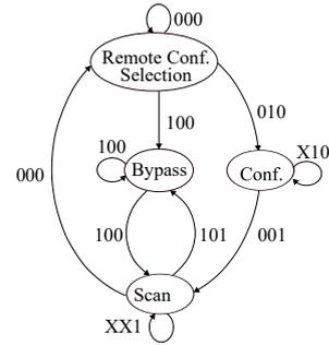
Fig. 3: Control states of proposed remote configuration architecture by considering  $(m_2, m_1, m_0)$  as input
