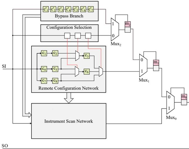
Fig. 2: proposed remote configuration architecture
