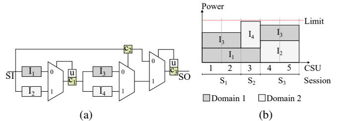
Fig. 1: (a) A small IJTAG network (b) The corresponding schedule based on power constraints and access requirements
